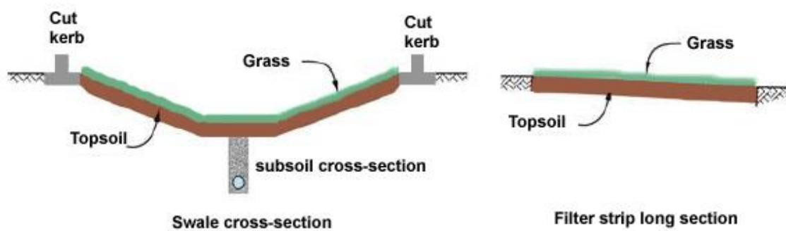
Swales and filter strips can treat runoff from impermeable hardstand ground surfaces in commercial, residential and industrial areas including roads and parking lot runoff. They provide aesthetic benefit.
