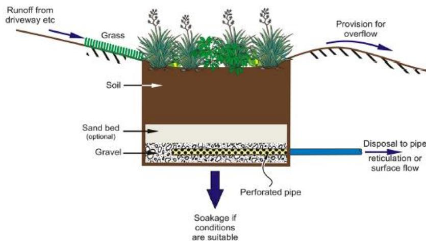
Raingardens can treat runoff from impermeable hardstand ground surfaces in commercial, residential and industrial areas, including parking lot runoff. Expected contaminant removal rates are as follows (ARC TP10, EPA 1999c):
