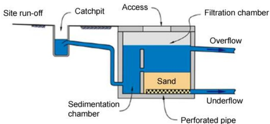
Filters are able to treat runoff from impermeable hardstand ground surfaces in commercial, residential and industrial areas. They provide significant peak flow or volume control. The most common filter is the sand filter. Expected contaminant removal rates for sand filters are as follows (ARC TP10, EPA 1999a):
