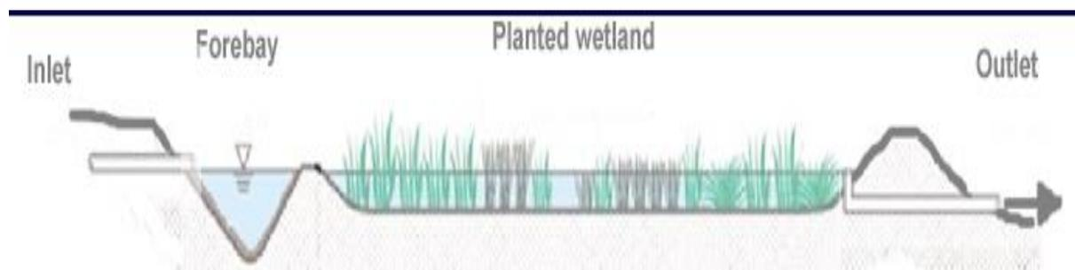
Wetlands can treat runoff from impermeable hardstand ground surfaces in commercial, residential and some industrial areas, including parking lot runoff. They are well suited for removal of sub 100-micron particulate matter and dissolved chemicals.
